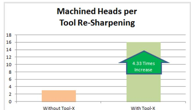
"We put in a TiCN coated reamer with the Tool-X and saw Ra numbers unlike anything we have ever seen. We started at 0.7 Ra on the first piece. We just pulled off our last piece (42 pieces later) and we are still holding at 1.2 Ra. This is unbelievable, our tool life more than quadrupled with that tool!"
